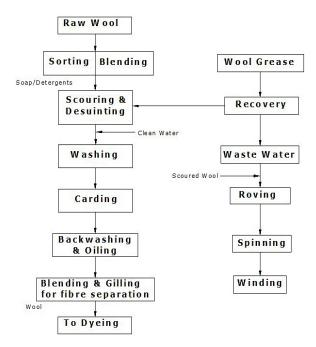
Figure 1. Process flow chart for wool scouring plant
